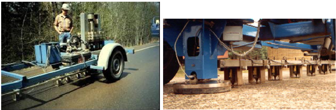
FIGURA 3.39: Falling Weight Deflectometer.
